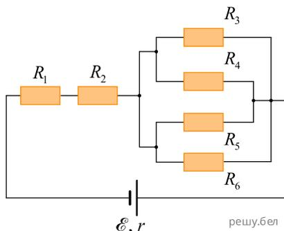
$$R_1 = R_2 = R_3 = R_4 = R_5 = R_6 = 10,0 \text{ Ом.}$$
